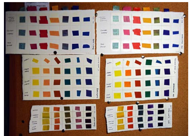
Experimental swatches testing fading and archival effects on different eras of paper with different glues and different varnishes.
